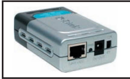
Photo 1 —The D-Link DWL-P50 is a ready-to-go module. Ethernet in, Ethernet out, and a choice between 12- and 5-VDC outputs.
