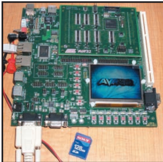
Photo 1 —Remember the old days when you plugged in a floppy disk to boot your computer? The STK1000 comes with the modern equivalent in the form of a 128-MB MMC flash card preloaded with Linux.
