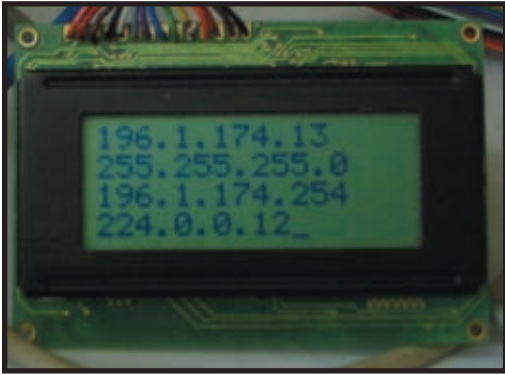
Photo 3 —This LCD module displays network information about the node such as the node IP address, netmask, gateway IP address, and group IP address.
