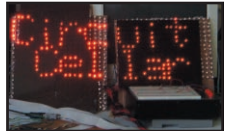
Photo 1 —These two 1'-squared panels were constructed out of a sheet of double-sided PC copper board. We placed makeshift red filters in front to enhance the contrast.
