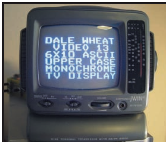
Photo 1 —The Video13 TV interface adds old-school charm to any project. What better way to get your message across than with chunky, monochrome, uppercase text?
