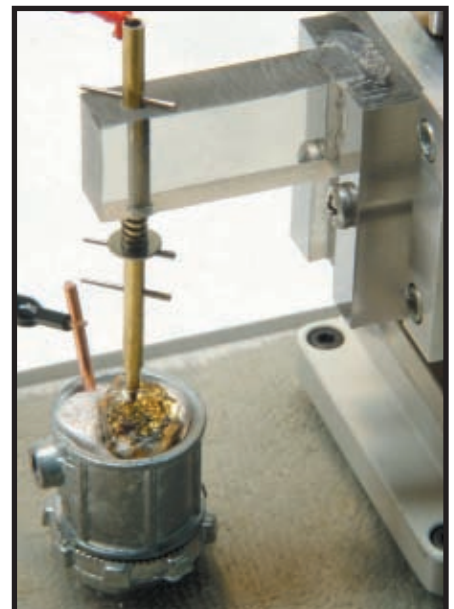
Photo 2 —The outer brass tube slides in the plastic holder with a spring for soft landings. The probe tips friction-fit in the end against the bottom taper pin. I cast a copper wire into the sample holder as an electrical contact.
