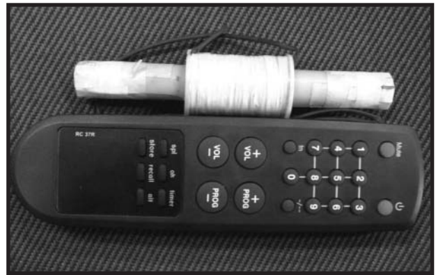
Photo 1 —Drop the batteries and go “green.” Simply connect my power generator to a regular TV remote control and shake.
