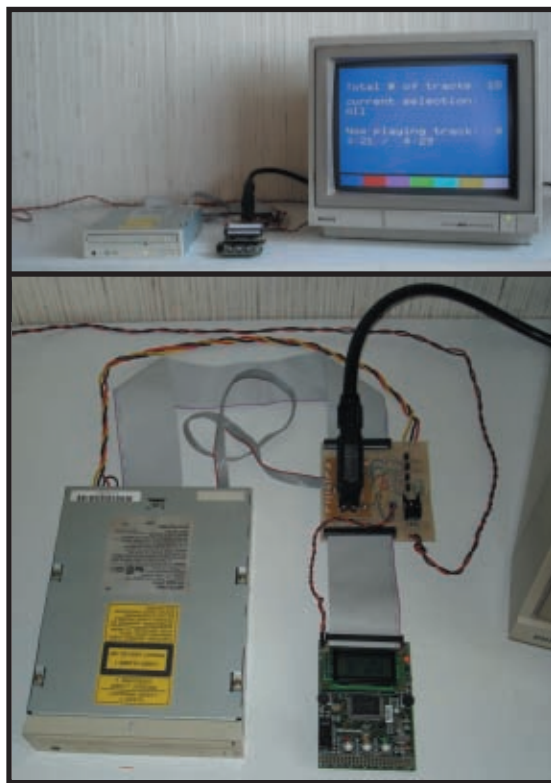
Photo 1 —The system includes a CD-ROM player, an M16C62P starter kit, an experiment board with the digital I/O-to-video level conversion, and an RGB monitor for displaying the video. The audio is rendered through the speakers in the monitor. Instead of the monitor, you can use the television in your living room.
